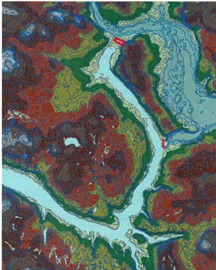
Figure 6: A renewable energy focus for the Mactaquac headpond. In this simplistic overview, we raise the issue of increased hydro power within the St John River watershed. Herein we roughly examined the effects of developing an earthen berm at the north end of the Mactaquac Arm with the intent of raising the headpond by 10 meters. This is not intended as a realistic proposal, but is instead a heuristic tool used to more fully highlight the key issues of concern surrounding the Mactaquac Dam. Preliminary analysis undertaken by Benjamin MacLellan, with support from Charles Bourque.
