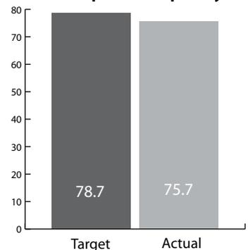
Capacity factor is the total amount of energy Point Lepreau produced during the year divided by the amount of energy the Station would have produced at full capacity.
