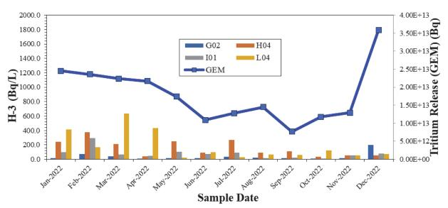
**Figure 4.14:** Gaseous H-3 Releases and Tritium (Precipitation) Results (Colour)
