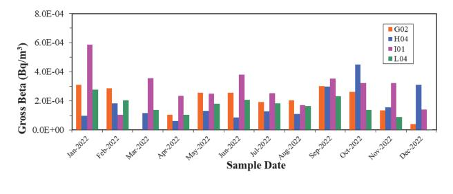
Figure 4.02: Gross Beta (Air Particulates) at Onsite Air Stations (Colour)
