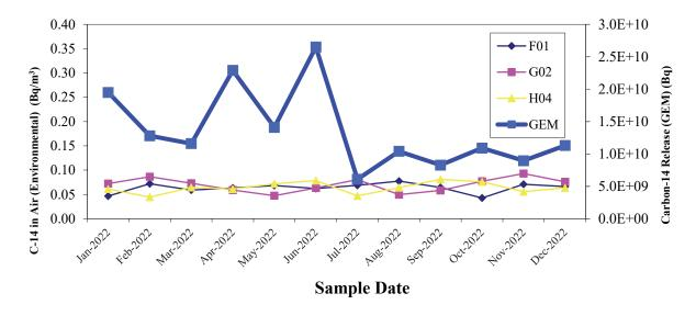
Figure 4.09: Gaseous C-14 Releases and C-14 (Carbon Dioxide) Results (Colour)
