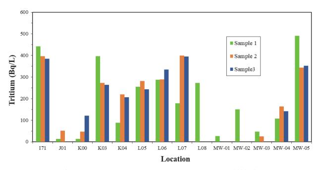
**Figure 4.15:** Tritium (Monitoring Well Water, Near Plant) 2022 (Colour)
