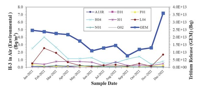
Figure 4.06: Gaseous H-3 Releases and H-3 (Water Vapour) Results (Colour)
