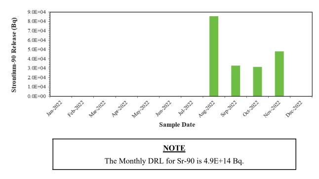
**Figure 4.19:** Liquid Sr-90 Releases for 2022 (Colour)
