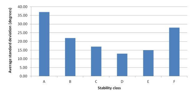
Figure 34: Average standard deviation of wind direction for each stability class
