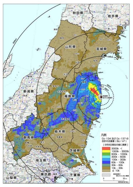
Figure 9: Ground contamination pattern at Fukushima [16]
