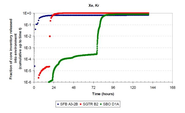
Figure 3: Noble gas cumulative release for the three unmitigated release categories
