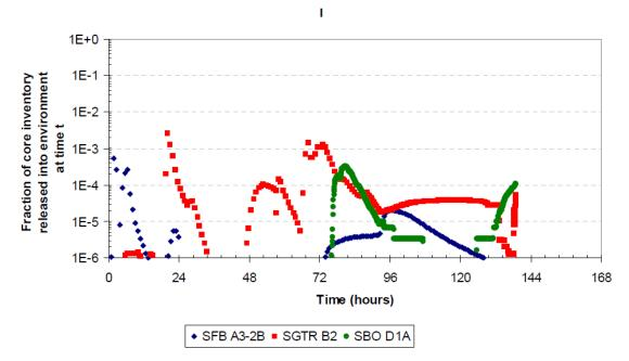
Figure 4: lodine and cesium release rate for the three unmitigated release categories
