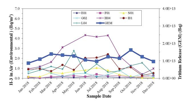
Figure 4.06: Gaseous H-3 Releases and H-3 (Water Vapour) Results
