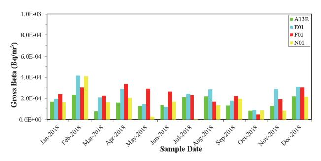
Figure 4.01: Gross Beta (Air Particulates) at Offsite Air Stations
