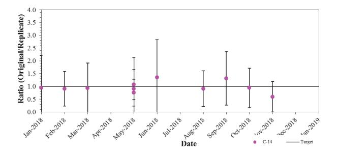
Figure 7.04: Carbon-14 Performance (Internal QA – duplicate/replicate)
