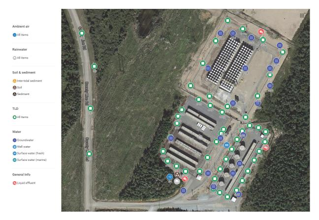
Figure 3.06: Environmental Monitoring at the Solid Radioactive Waste Management Facility (SRWMF)
