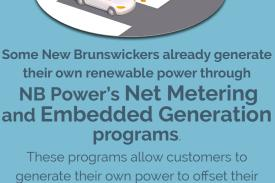
consumption while remaining connected to the distribution system. This ensures they can meet their electricity demands when their generation unit cannot.
